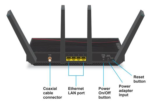
Figure 3. Modem router rear panel
