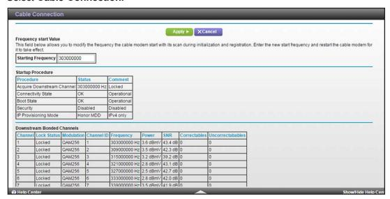
The Startup Procedure section displays the initialization progress. The page also displays the status of all downstream and upstream channels. (You must scroll down to view all the channels.) The number of downstream and upstream channels that are locked depends on the number of channels that your Internet provider uses.
